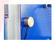
MEASUREMENT AND CALIBRATION OF TOOL LENGTH Carries out automatic control of tool length and allows, when starting work, to quickly enter data on the table surface (Z = 0) and material height.
