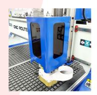
The design of the spindle is based on the best design solutions of the world's leading manufacturer of spindles - HSD (Italy). High rotational speed (18.000 rpm) and optimum power (6 kW) make it possible to process parts made of wood, as well as chipboard, MDF, plastic, acrylic glass and other materials for the manufacture of furniture, doors, advertising and souvenirs with high quality.
